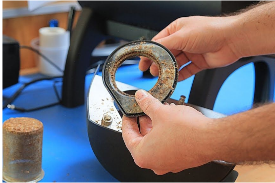
Remove rubber gasket, brush off the chaff
